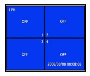
The DVR system can display 4 camera feeds in one picture (Quad Mode).
